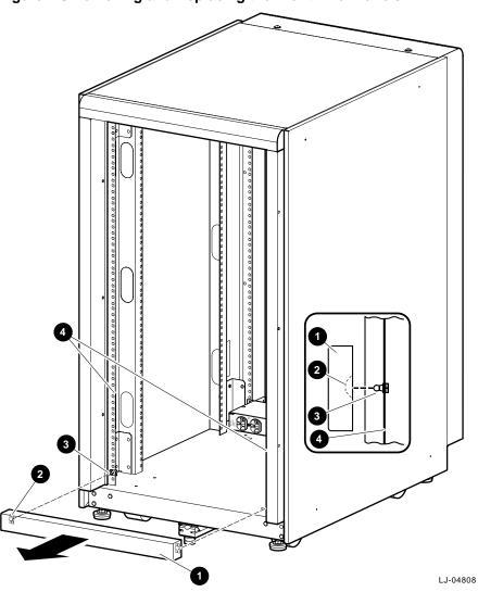
Figure 2-5 Removing and Replacing the Front Filler Panels
